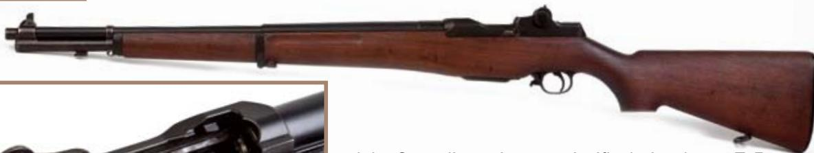
*John Garand's semi-automatic rifle design, here a T3E2, accepted an en-bloc clip that could be fed either way.*
