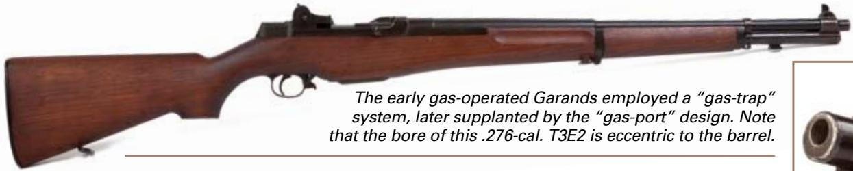
*The early gas-operated Garands employed a "gas-trap" system, later supplanted by the "gas-port" design. Note that the bore of this .276-cal. T3E2 is eccentric to the barrel.*
