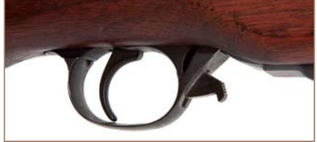
*On the T3E2, the safety was in the front of the trigger guard, but not of the shape as finally adopted in 1936.*
