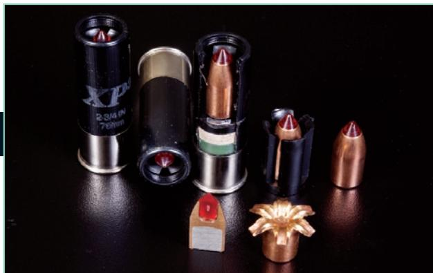
*The gilding metal nose of Winchester's XP<sup>3</sup> slug splits along pre-stressed lines into six petals. The 12-ga., 300-gr. projectile expanded to 0.99", and its retained weight was 294 grs. It delivered the highest muzzle velocity.*
