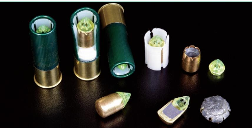
*The Remington AccuTip Bonded Sabot Slug (top, and l.) is the newest of the class—and the most unusual. Its huge polymer tip has a series of holes in its ogive that change the drag forces on the slug. Remington engineers did this to change the center of pressure on the slug. The jacket is made from cartridge brass—like Golden Saber pistol bullets—while the core is of soft lead. In the author's tests, the 12-ga., 385-gr. projectile expanded to 0.97" and had a retained weight of 370.5 grs.*
