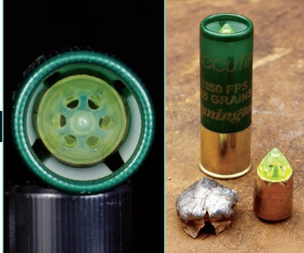
of pressure. Dennison tried several designs before finding the configuration that gave him the best accuracy. The added drag reduces the ballistic coefficient, but the theory is that a slightly flatter-shooting slug is of no use if the accuracy is not there.
