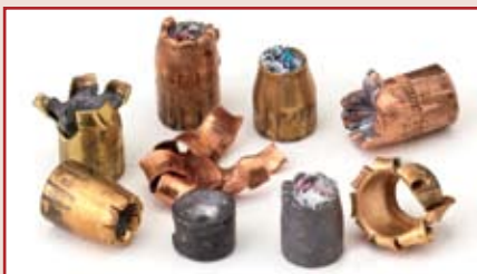
Traditional hollow-point handgun bullets typically produce erratic, if any, expansion when clogged by clothing (l.). Critical Defense's FTX bullet (center) eliminates this variable, resulting in reliable, consistent expansion (r.).
