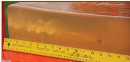
Winchester's Bonded PDX1 (l.) met the FBI requirements for penetration, which calls for at least 12" after encountering barriers (center). Typical expansion is 1.5 times the original diameter (r.), and weight retention is near 100 percent.
