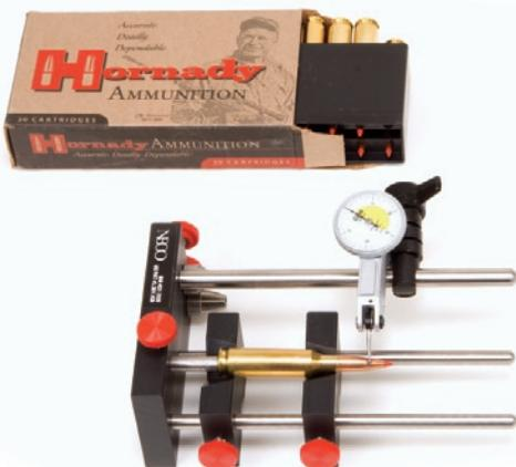
able to attribute these instances to barrels with either short throats or tighter-than-normal bores. In some cases, the barrels had bores as much as 0.002" tighter than the nominal groove specification of 0.264". According to Dave Emary, 6.5 Creedmoor barrels should measure 0.257" and 0.264" for the land and groove diameters, respectively.
