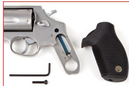
*The frame extension, containing the gun's coil mainspring, rests within the Judge's rubber one-piece grip.*
