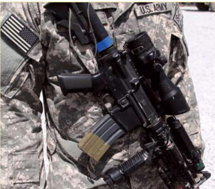
*The well-outfitted M4 carbine today is likely to have a variety of optical and shooting aids—in this case a AN/PAQ-4 laser designator, Trijicon ACOG 4X sight and GripPod combination vertical foregrip/bipod.*
